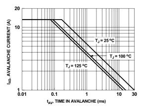
Figure 9. Unclamped Inductive Switching Capability
