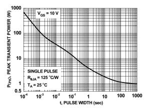
Figure 12. Single Pulse Maximum Power Dissipation
