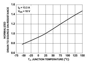
Figure 3. Normalized On-Resistance vs Junction Temperature
