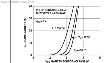
Figure 5. Transfer Characteristics
