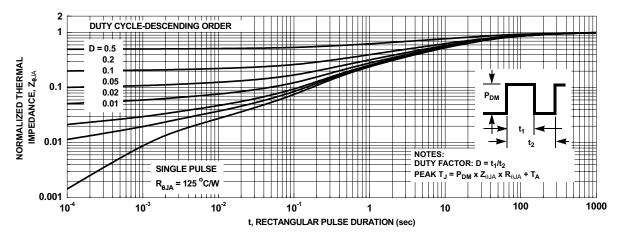
Figure 13. Transient Thermal Response Curve
